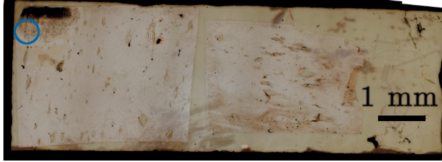
Figure 4.9: Microscope image of the CNT samples after a few rounds of experiments. The top left corner of the sample has been blackened after extended exposure to THz radiation. The blue circle depicts the rough position and size of the THz which caused the damage. The THz polarization was parallel to the short edge of the sample.
