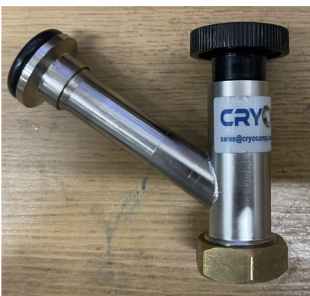
Figure D.1: Specialized Cryomech vacuum jacket adapter. Bronze nut tightens O-ring onto liquifier vacuum jacket port. Thumbscrew (black) is used to turn screw threads into the valve plug, pulling this thumbscrew out removes the plug and allows the system to be pumped down. It may be helpful to wedge something between the thumbscrew and port during pumping to ensure the plug stays removed.
