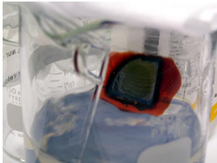
Figure 3.3 Close-up pictures of the spray etch setup. The AlGaAs etch-stop layer is reached first at the center of the wafer where the etch rate is highest. Over-etch of about 1 hour is needed in order to complete etching the whole wafer.
