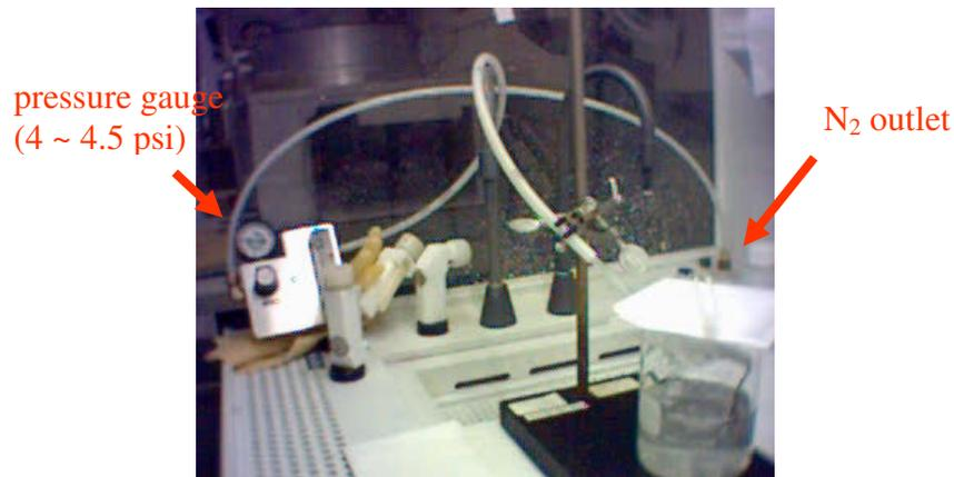
Figure 3.2 Spray etch setup. Pressure is maintained at 4 ~ 4.5 pounds per square inch (psi).
