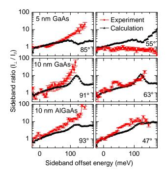
Figure 4.12: Comparison of experiment and theory. The ratio  $I_{\perp}/I_{\parallel}$  is compared in all three quantum wells at different lattice angles. The non-Abelian Berry connection is responsible for the qualitative agreement. The quantum theory of sidebands only includes macroscopic dephasing, no k- or t-dependent scattering. Comparing intensity ratios instead of absolute intensities cancels out some of the complicated scattering behavior.
