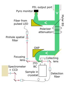
Figure 3.10: The optical schematic of a driven absorption experiment. This measurement combines the DT measurement with THz illumination. Instead of the tungsten-halogen lamp, however, an electronically-switched LED provides the NIR power only while the FEL is lasing.
