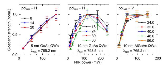
Figure 4.4: The NIR power dependence of HSG in the three samples. (left) The sideband signal in the 5 nm GaAs sample is almost exactly proportional to the NIR power for sideband orders between 8 and 14. (center) The sideband signal in the 10 nm GaAs sample, however, has a strong peak at 125 mW for orders between 18 and 36, but it departs from linear at around 50 mW. (right) The sideband signal in the 10 nm AlGaAs sample actually plateaus at 50 mW.
