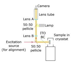
Figure A.2: The optical setup for the sample imaging camera.
