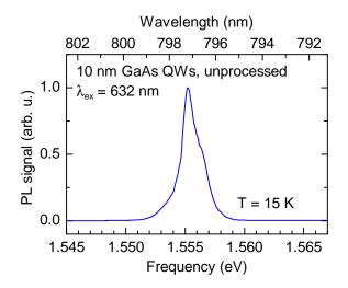
Figure 3.2: A PL spectrum from undoped quantum wells (QWs) as-grown. A HeNe laser excites the PL,  $\lambda_{ex} = 632$  nm. The single peak results from radiative recombination of heavy hole excitons. The small shoulders in the peak result from well-width fluctuations in the QWs distributed across the ten-well stack and the 200  $\mu$ m laser spot. At 15 K, there is no significant population of light hole excitons about 10 meV above the heavy hole exciton peak.
