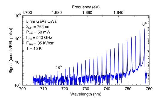
Figure 3.8: Example sideband spectrum measured by the CCD. Sidebands of order  $6 \le n \le 48$ , spanning 40 nm, can be observed in four images covering 20 total FEL pulses, or 800 ns of THz power. The strongest four sidebands spill a little bit out of their pixels during readout, but 30 dB down from the peak. Overlap between this spectrum and the PMT spectrum in Fig. 3.6 to calculate the efficiency of these sidebands as well.
