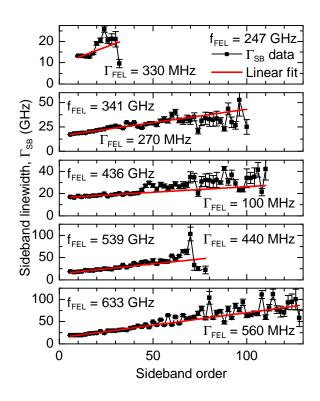
Figure 3.14: The fits of the linewidths for various FEL frequencies. The black squares are the linewidths from fitting sideband peaks with Gaussian functions, and the reported  $f_{\text{FEL}}$  is measured from sideband spacings as discussed in Fig. 3.13. The red line is a linear fit to linewidths as a function of order. The y-intercept for all but the 247 GHz spectrum is consistently 15 GHz. The slope is the linewidth of the FEL,  $\Gamma_{\text{FEL}}$ , reported in each subfigure.
