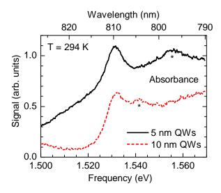
Figure 2.4: Room temperature absorption spectra. The heavy hole exciton lines still dominate the absorption spectra of both samples, but the light hole excitons (denoted by the \*), are still observable. The half linewidth of the heavy hole exciton line is 4 meV in the 5 nm GaAs QWs and 5 meV in the 10 nm AlGaAs QWs. The data was published in [4]. Copyright 2013 by the American Physical Society.
