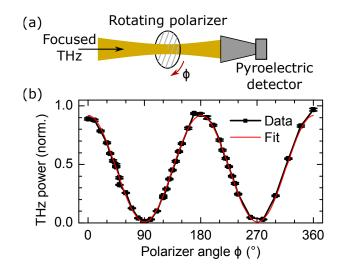
Figure 4.5: Measuring THz polarization. (a) A wire grid polarizer is mounted to a rotatable stage and placed at the focus of the THz beam. A fast, horn-coupled pyroelectric detector is placed immediately behind the wire grid. (b) The THz power measured behind the polarizer as it was rotated. The signal was normalized the the signal when the polarizer was removed. The peaks at 0 and 180° and minima at 80 and 270° reveal that THz beam is > 99% horizontally polarized.
