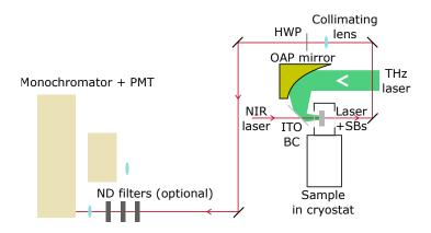
Figure 3.5: The optical schematic for sideband PMT detection path. Sidebands are created with a similar beam profile as the NIR laser. They are collimated by a lens after the sample, and the polarization is rotated using the HWP for maximum grating efficiency in the monochromator. Because PMT is easily saturated, calibrated neutral density (ND) filters allow for measurements of the NIR laser line and the strong low-order sidebands.
